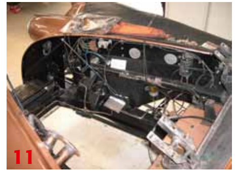
The engine bay with repairs to the inner wing invisible and many of the minor components replaced ahead of refitting the engine
