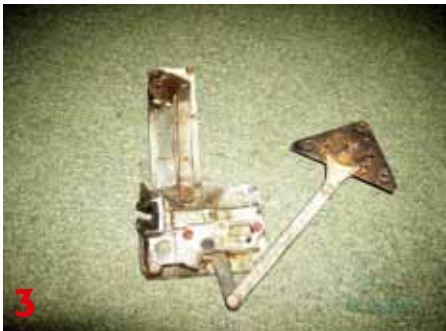
Even though this was only a partial rebuild, much detail work was needed. This is the lock mechanism from the offside door about to be refurbished, one of many sub-assemblies given attention
