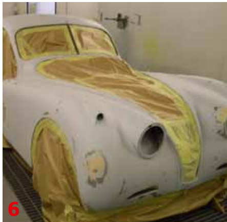
Unlike a full restoration, where the bare bodyshell would be painted, LWK 707's interior remained in situ, requiring Alex to mask off all areas to be protected from overspray. Although the final coats would be cellulose, to prevent sinking and reaction a non-permeable epoxy coat was applied first, followed by a two-pack primer
