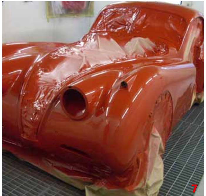
A dramatic stage in the painting process was when next this gloss red oxide paint with a matt controller was applied to the primed body
