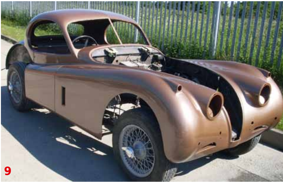
This is the car just after the basic painting process had been completed, ready for fitting-up with the engine, transmission and all the other items which had been removed. Note the driver's door – at first it was thought that the original was a write-off, but it was retrieved along with its trim panel and wood
