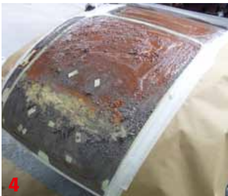
Meanwhile the repaired bodyshell was being made ready for the paintshop, with localised stripping revealing old minor repairs. The old paint, most of it dating back to 1952, was then stripped from the entire body; here the bootlid is being tackled
