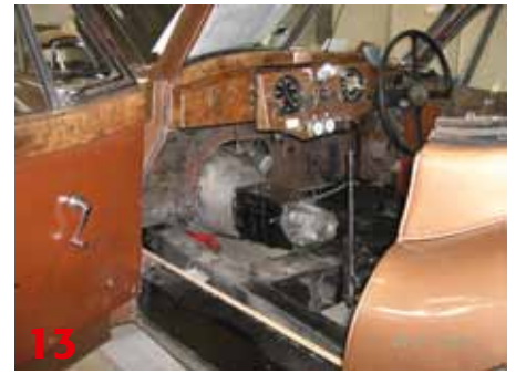
The gearbox, refitted along with the engine, seen from the cockpit. The original plywood floor was found to be in good condition
