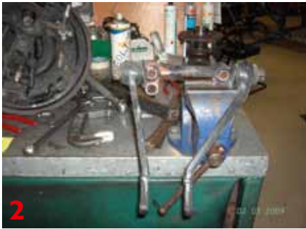
The wishbone front suspension was largely undamaged but was stripped down, crack-tested, and rebuilt with new bushes and balljoints as required
