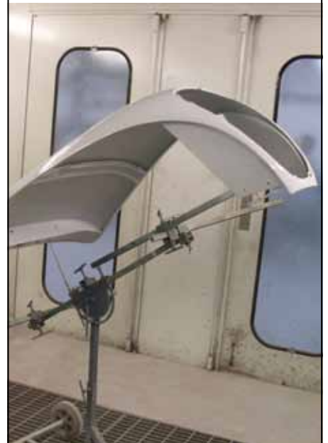
The rear wings – even the undamaged nearside one – had to be removed for painting separately (above), as a beading lies between wing and body that can't be masked off satisfactorily. The same applied to the bonnet (below) which also cannot be painted while on the car
